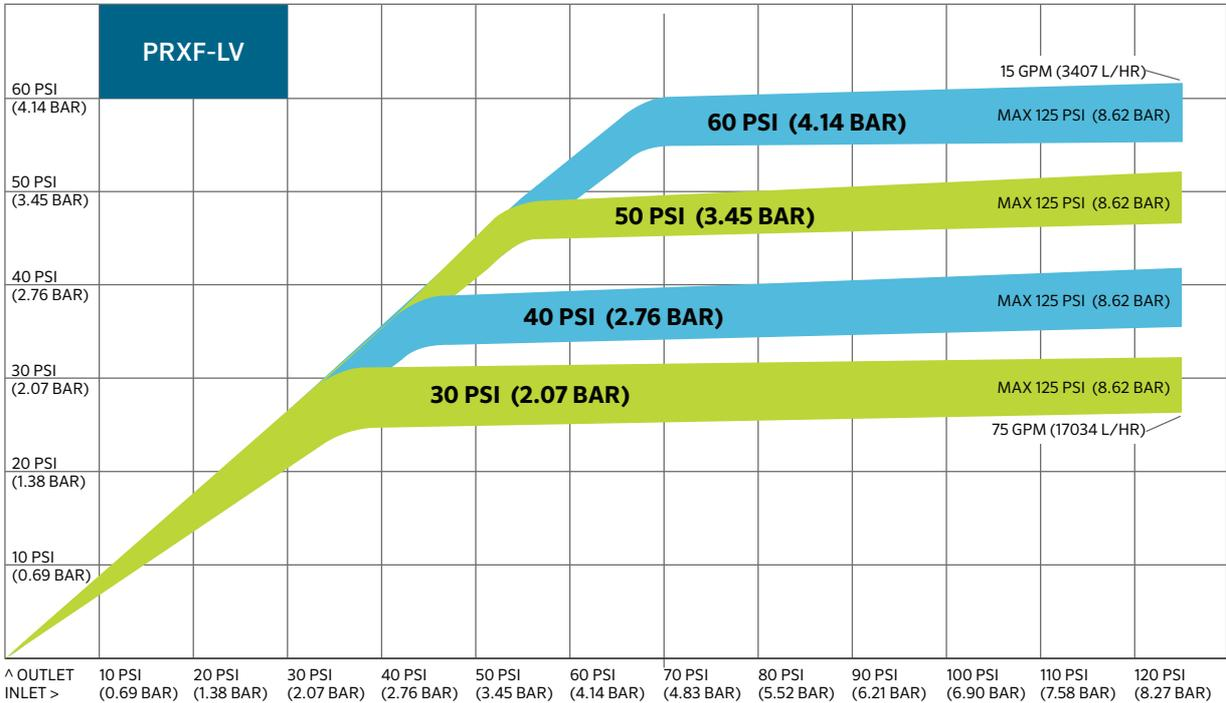
Every pressure regulating extended flow limit valve is designed to operate at a minimum and maximum inlet pressure and a predetermined flow range. This regulation performance curve illustrates how the PRXF-LV will perform within the range of inlet pressures and flows.
