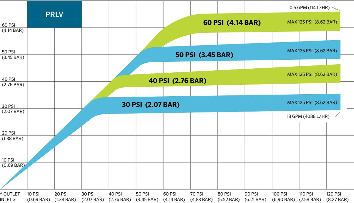
Every pressure regulating limit valve is designed to operate at a minimum and maximum inlet pressure and a predetermined flow range. This regulation performance curve illustrates how the PRLV will perform within the range of inlet pressures and flows.
