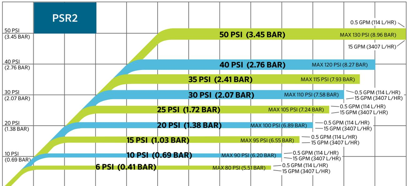
In this chart, the band for the 30 psi (2.07 bar) model shows the performance at various flows. At the lowest flow (0.5 gpm or 114 L/hr), the regulator will maintain an actual outlet pressure slightly higher than 30 psi (2.07 bar). In contrast, at the highest flow (15 gpm or 3407 L/hr), the actual outlet pressure will be slightly lower than 30 psi (2.07 bar)\*.
