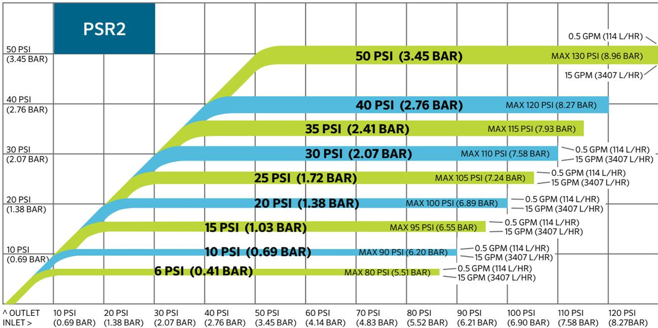
Every pressure regulator is designed to operate at a minimum and maximum inlet pressure and a predetermined flow range. This regulator performance curve illustrates how the PSR2 will perform within the range of inlet pressures and flows.
