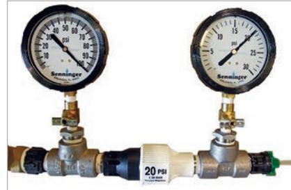
*If your irrigation dealer has a regulating testing device, you can also check the readings on a new pressure regulator that matches the model you are testing.*
