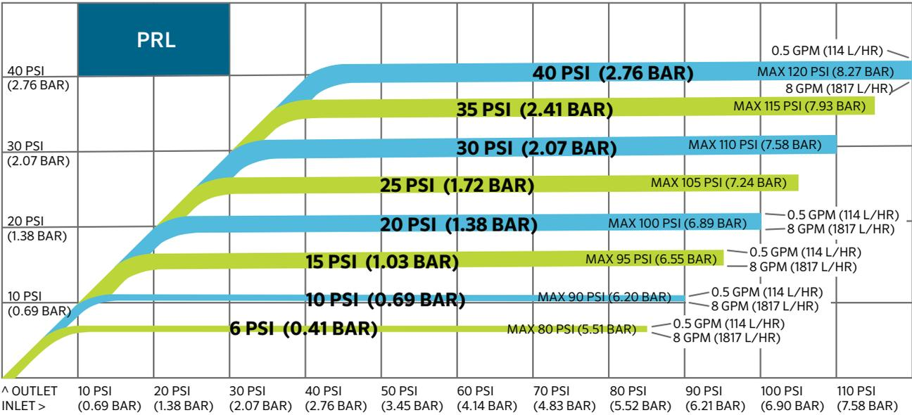
Every pressure regulator is designed to operate at a minimum and maximum inlet pressure and a predetermined flow range. This regulator performance curve illustrates how the PRL will perform within the range of inlet pressures and flows.
