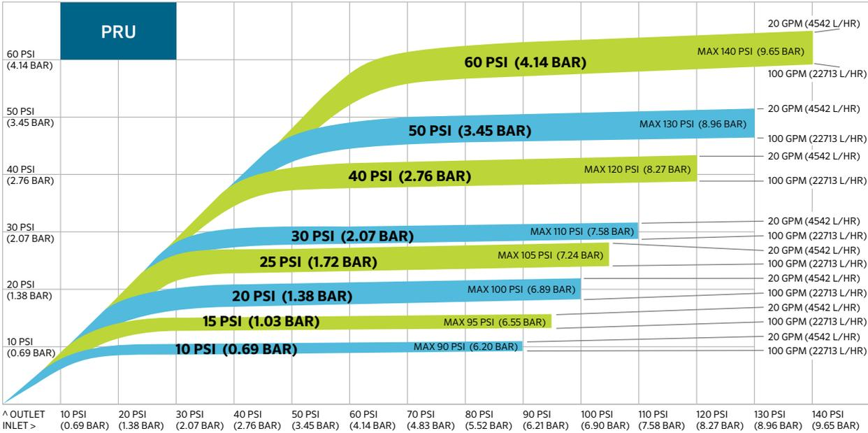
Every pressure regulator is designed to operate at a minimum and maximum inlet pressure and a predetermined flow range. This regulator performance curve illustrates how the PRU will perform within the range of inlet pressures and flows.
