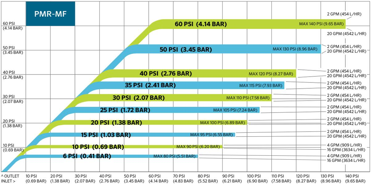
Every pressure regulator is designed to operate at a minimum and maximum inlet pressure and a predetermined flow range. This regulator performance curve illustrates how the PMR-MF will perform within the range of inlet pressures and flows.
