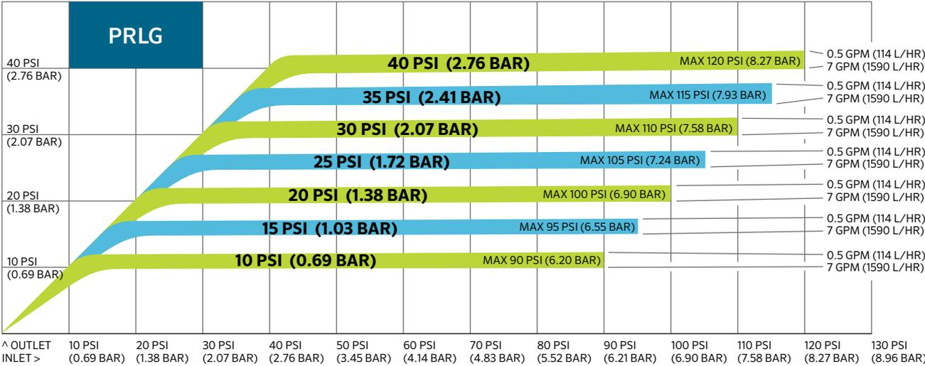
Every pressure regulator is designed to operate at a minimum and maximum inlet pressure and a predetermined flow range. This regulator performance curve illustrates how the PRLG will perform within the range of inlet pressures and flows.
