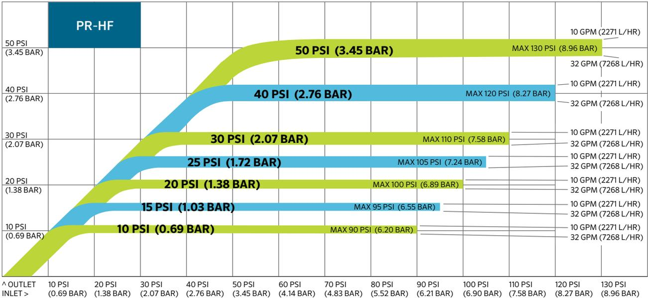
Every pressure regulator is designed to operate at a minimum and maximum inlet pressure and a predetermined flow range. This regulator performance curve illustrates how the PR-HF will perform within the range of inlet pressures and flows.
