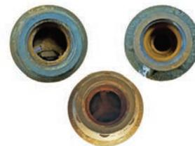
*Inlet and outlet of worn pressure regulators.*
